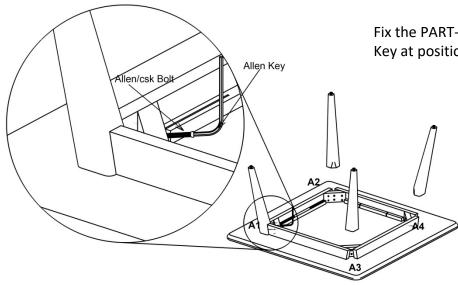
Fix the PART-B (leg) with Allen Bolt using Allen Key at position A1,A2,A3 & A4 as shown in Fig.
