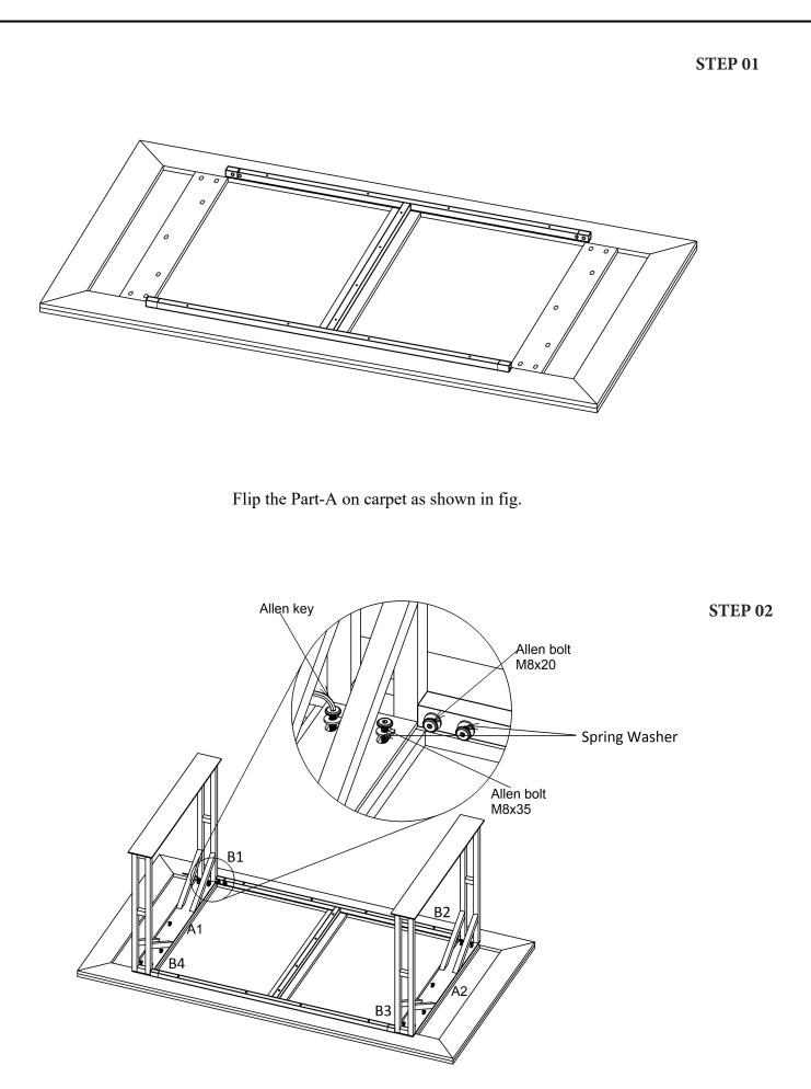
Now fix Part-B with Part-A from allen bolt M8x35 mm at position A1,A2, and from allen bolt M8x20mm at position B1,B2,B3 and B4 including spring washer using allen key as shown in fig.
