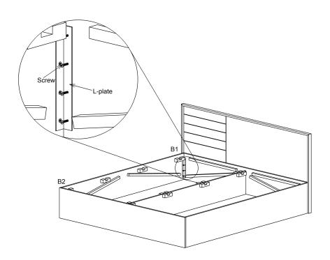
Now fix Part -C(Side panel) with Part-A (Headboard) and Part-H(Footboard) by L-plate and screws 16mm at position B1 and B2 respectively as shown in fig.
