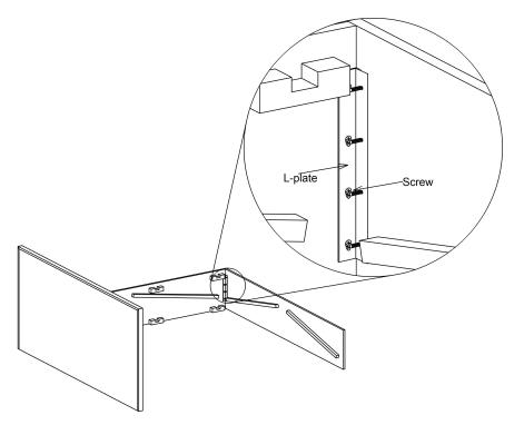
Fix the Part-H (Footboard part) and last assembled part with L-plate and screws as shown in fig.
