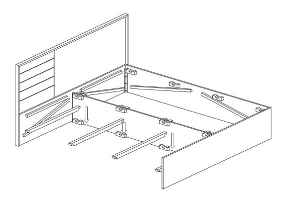
Now place Part-C (Battens) at bottom U-block as shown in Fig.
