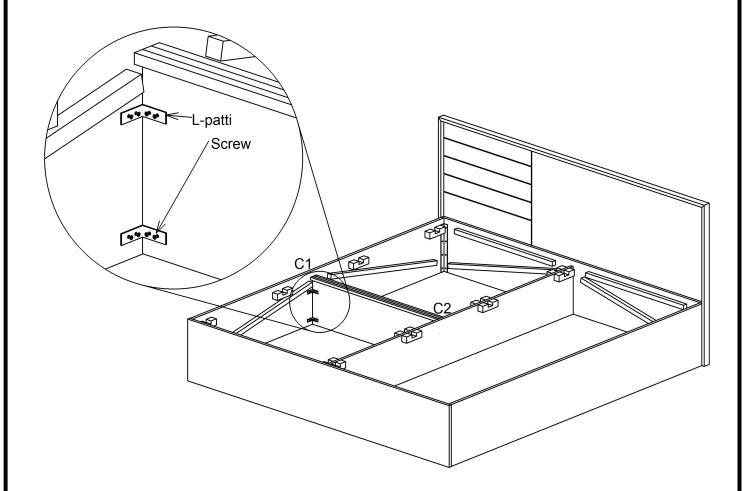
Now fix Part-G(middle partition) using L-patti and screws at position C1 and C2 as shown in fig.
