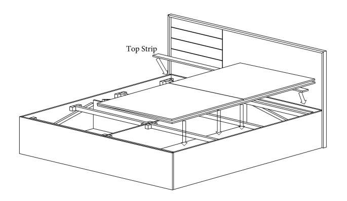
Now place Part-B (Top strip) and Part-I(Top panel) at last assembled as shown in Fig.
